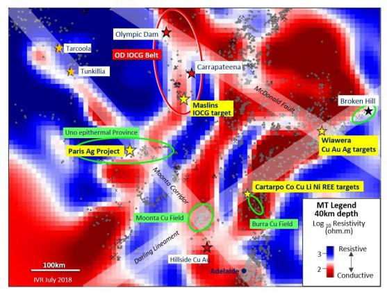
Figure 2: Government Magneto-Telluric ("MT") image of modelled rock resistivity at 40km depth with metal occurrences shown as grey dots & cross-picks. Major mines and selected projects are labelled in white with black stars. Key Investigator prospects and targets are added as yellow stars and labels. (MT & occurrence image source: Department of Energy & Mining SARIG Database).
