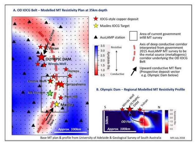
Figure 3A: Olympic Dam IOCG Belt – MT resistivity plan at 35km depth slice modelled from coarse first-pass AusLAMP data showing locations of IOCG deposits & prospects; axis of the OD MT Conductive Corridor and traces of interpreted MT flares.
