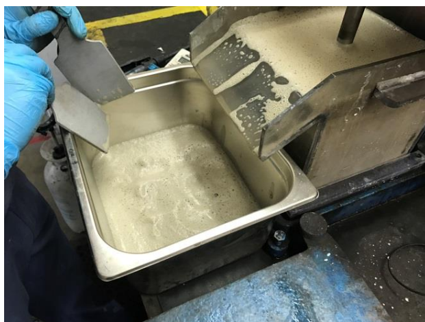
Photo 3: Flotation test on P 80 53µm grind size
