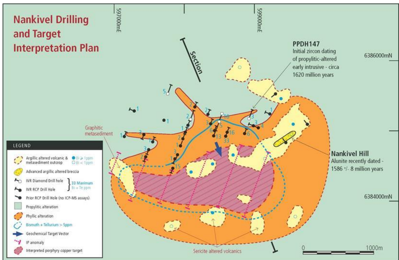
Figure 2: Plan showing the targeting ingredients for the interpreted Nankivel porphyry copper target
