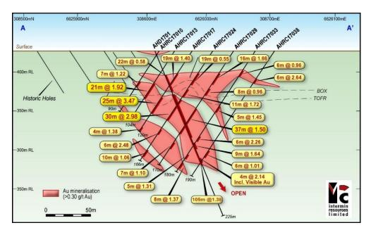
Figure 6: Anthill prospect cross section with 2017 drilling results
