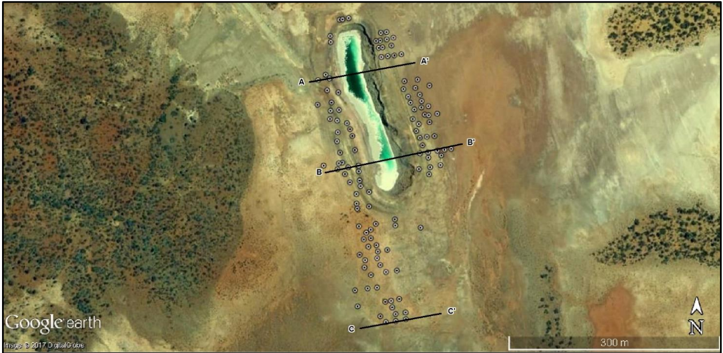
Figure 2: Goongarrie Lady drill collar and cross section location plan over historic open pit
