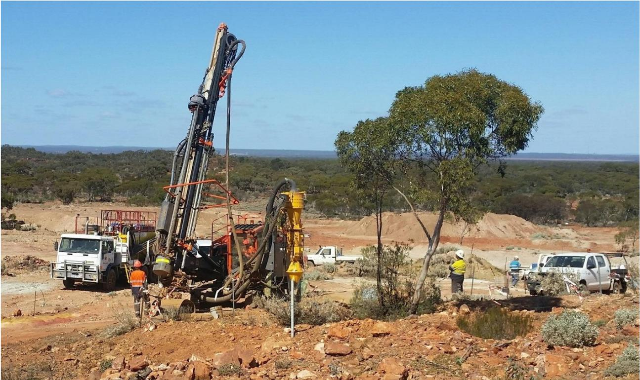
**Figure 3: Commencement of grade control drilling in the Regal area of Boorara**
