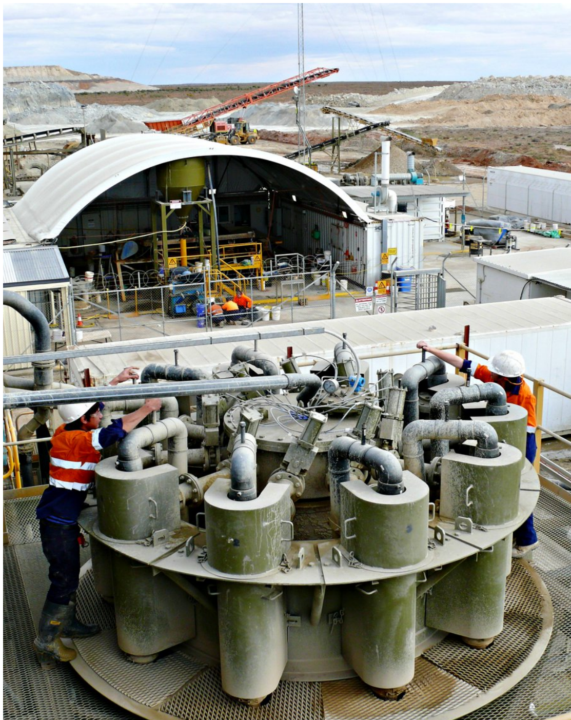
Final commissioning adjustments being made to the newly installed cyclone by one of Havilah's process engineering employees
