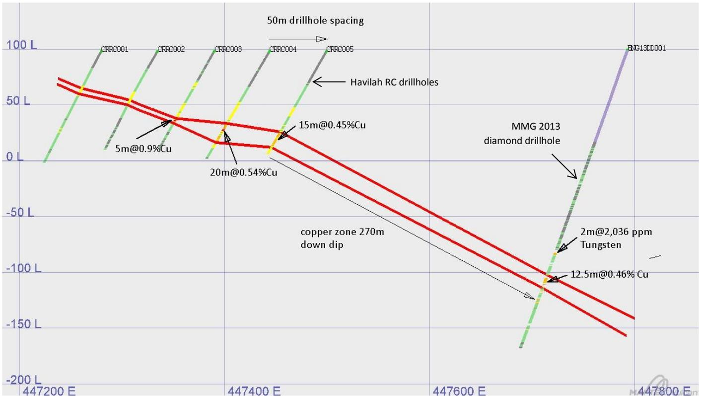
Havilah drillholes CRRC 1 to 5 were all sited to intersect the interpreted copper mineralised horizon (defined by the red lines) that was projected some 300-400 metres up-dip from the earlier MMG diamond drillhole BNG13DD001.
