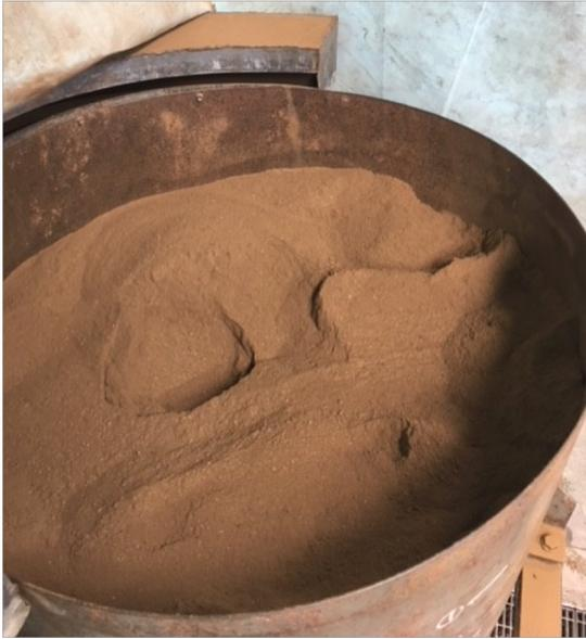
Pilot Plant feed ore, containing 1.02% TREO, including 0.43%  $\text{Nd}_2\text{O}_3 + \text{Pr}_6\text{O}_{11}$
