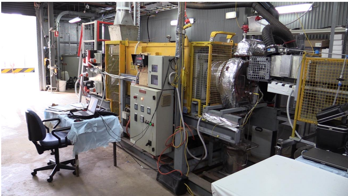
Figure 1 Hydrometallurgy Pilot testing - Acid Bake Kiln
