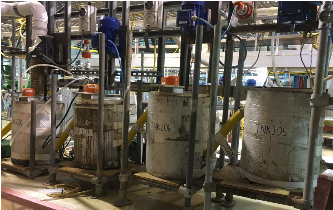
Figure 2 Hydrometallurgy Pilot testing – Water Leach Circuit
