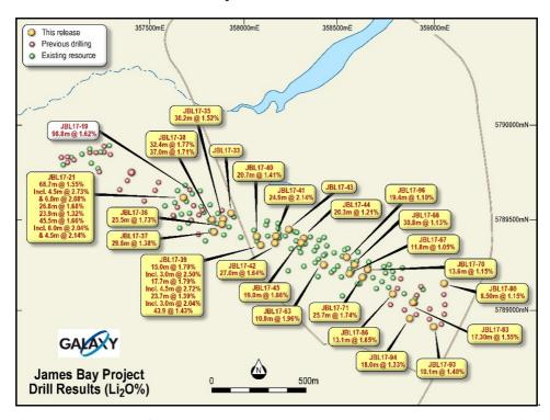
Figure 2: Plan view of collar positions (new assay in yellow, previous 2017 assays in red, existing resource collars in green).
