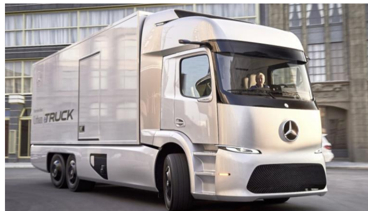
Daimler (Mercedes-Benz) Electric Truck (212kWh battery)
