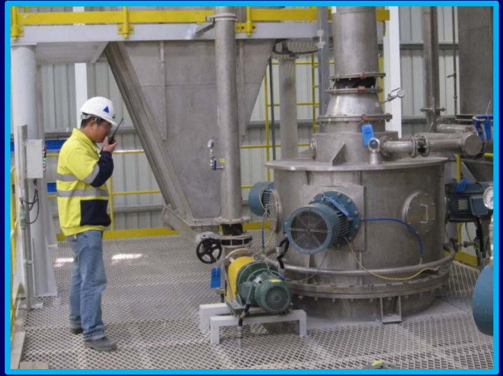
First material being micronised during hot commissioning
