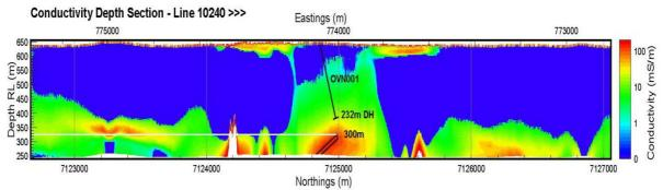
Figure 3: Position of Rio Tinto drilled hole at Oval overlaid on VTEM data. Note position of conductor below termination of OVN001.
