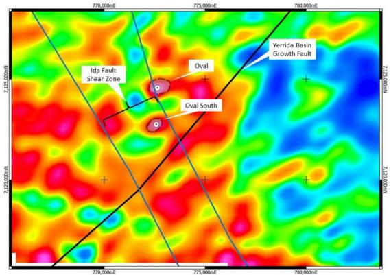
Figure 4: Oval and Oval EM anomalies, overlaid on gravity gradiometry data. Note the location of the Ida Fault Shear Zone and Yerrida Basin Growth Fault, focusing potential metal rich fluids GTE ASX Announcement 4 October 2023).
