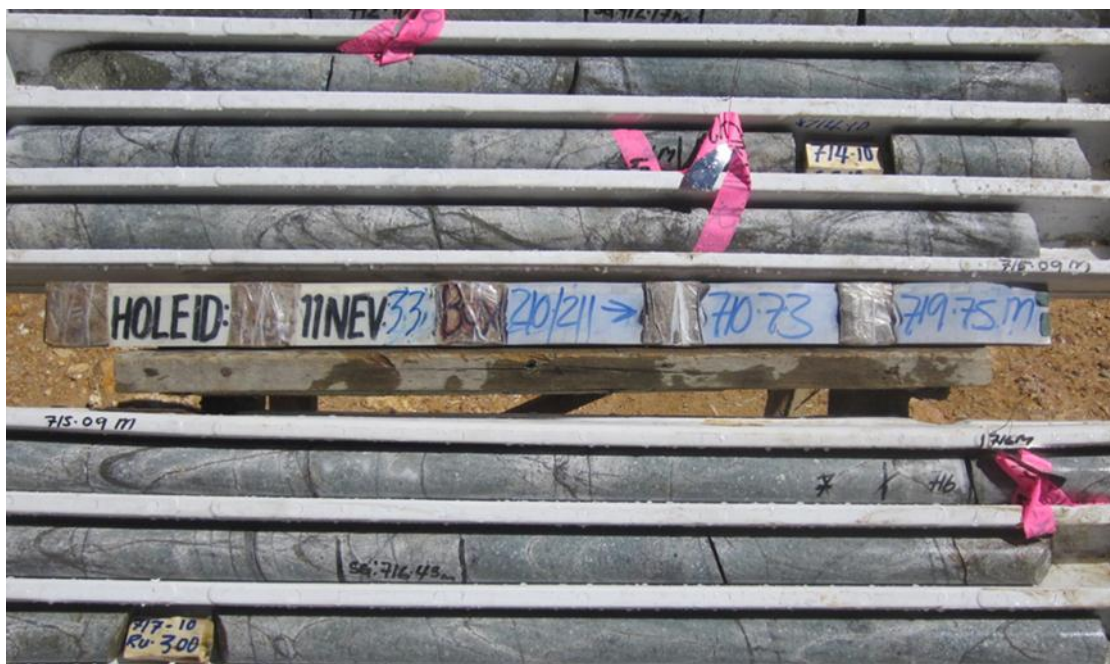
Figure 3 - NEV033 Drill Core Assay Result 714m to 716m: 2m at 1.7 g/t Au, 0.15% Cu (this lies within 22m section 706m to 728m averaging 0.81 g/t Au, 0.12% Cu)
