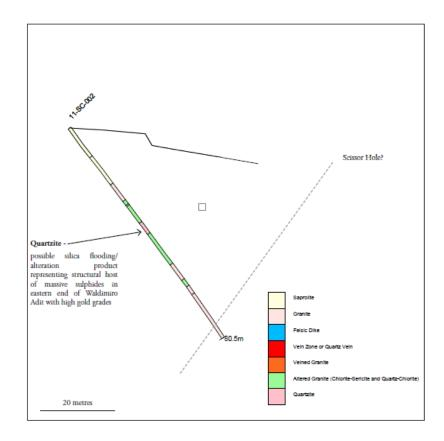
FIGURE 2 Section through 11-SC-002 facing west, showing with proposed scissor hole, if warranted following drillholes 11- SC-005 and 11-SC-006
