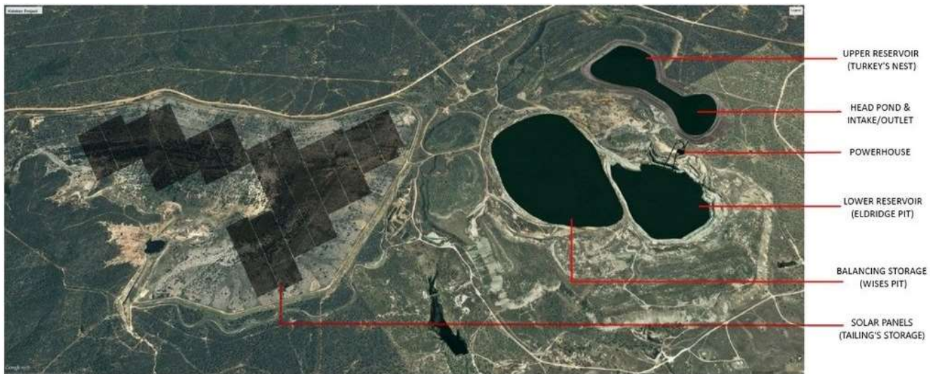
The Kidston Renewable Energy Hub: 50MW Solar Project and the 250MW Pumped Storage Hydro Project
