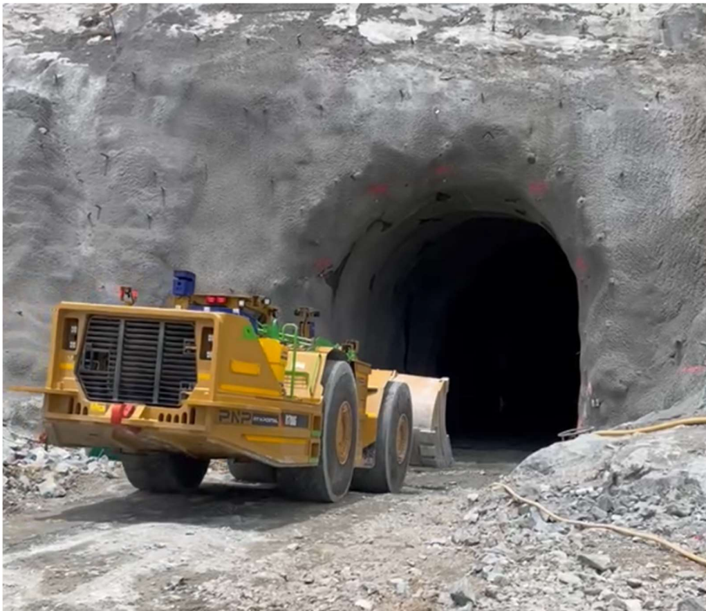
Figure 4: Underground Loader mucking out after blasting
