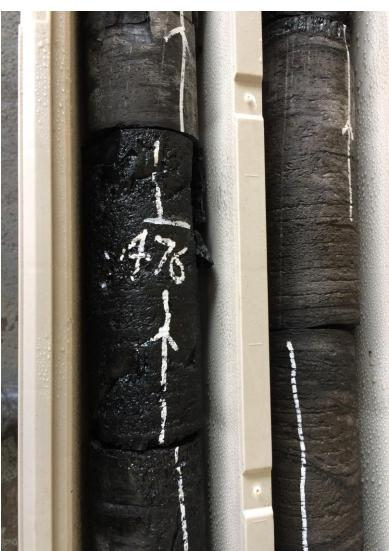
Coal core and carbonaceous shale samples from upper Reid's Dome Beds within Nyanda-4
