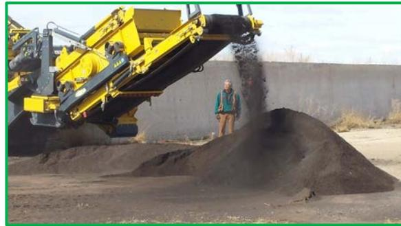
**Fernie rock phosphate being processed by Keestrack “Destroyer 1011” crusher and pulverizer**
