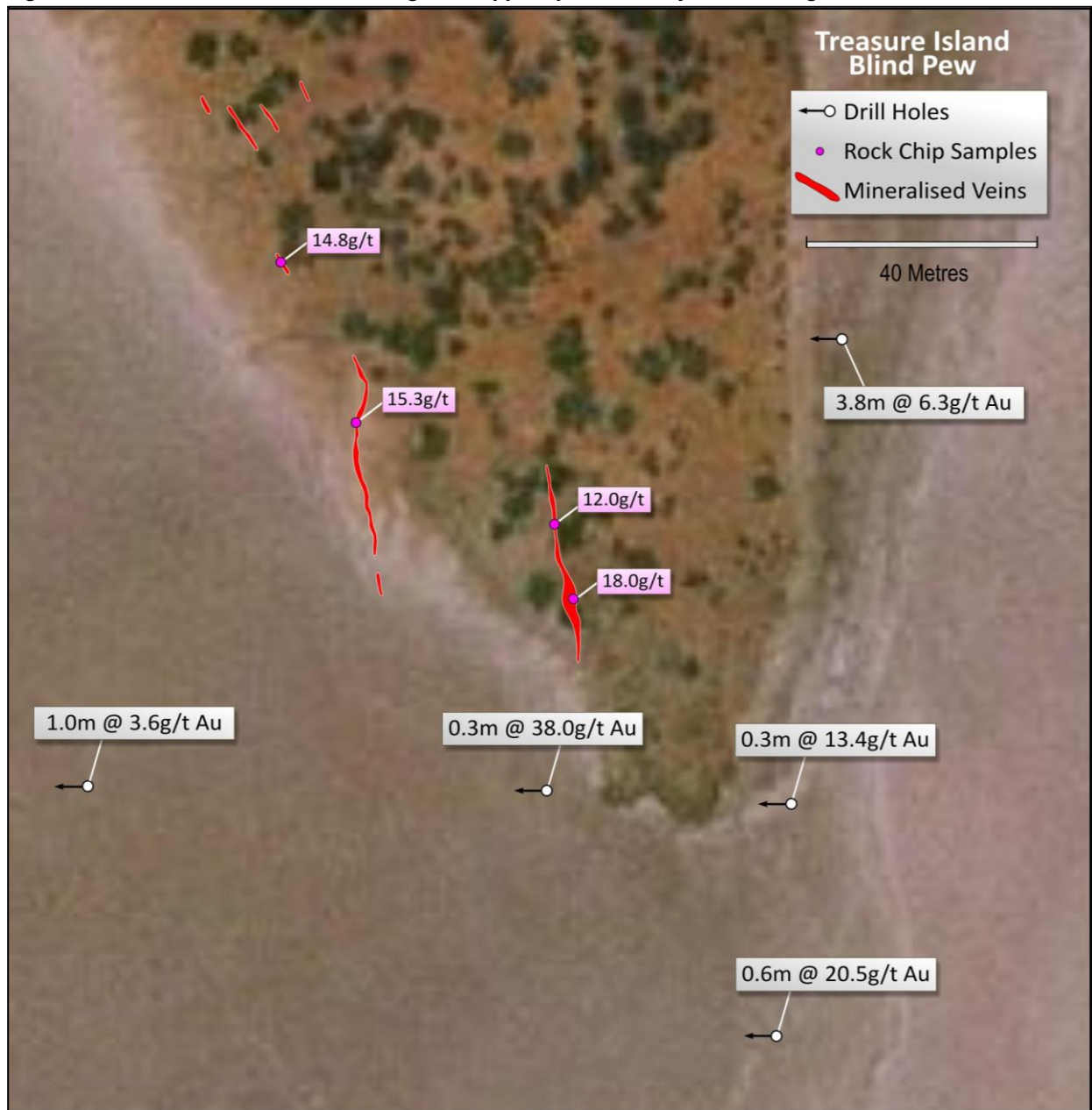
Figure 6: Plan view of Blind Pew showing the mapped quartz vein system and significant drill results.
