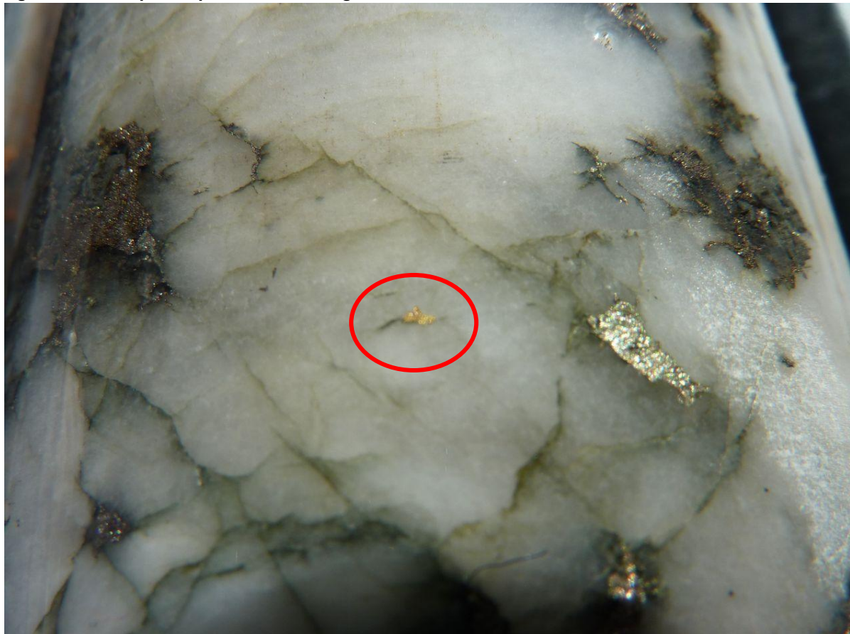
Figure 5: Close up example of fine visible gold seen in drill core from BDDD011 shown above.
