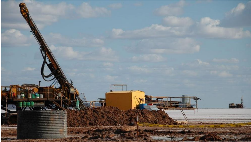
Figure 7: Diamond drill rig on lake bed at Treasure Island with aircore rig in the background.
