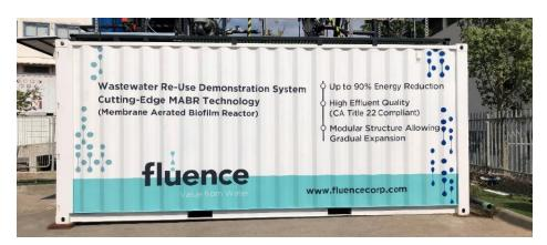
Deploying the MABR Unit will pave the way for Fluence to test and achieve California's strict Title 22 requirements for water reuse and allow observation of the plant in operation. MABR systems represent a cost-effective decentralized treatment for reuse, as well as being an affordable upgrade to a large existing installed base of conventional treatment plants aiming to achieve effective nitrogen and phosphorous removal.
