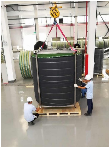
First completed MABR Module
