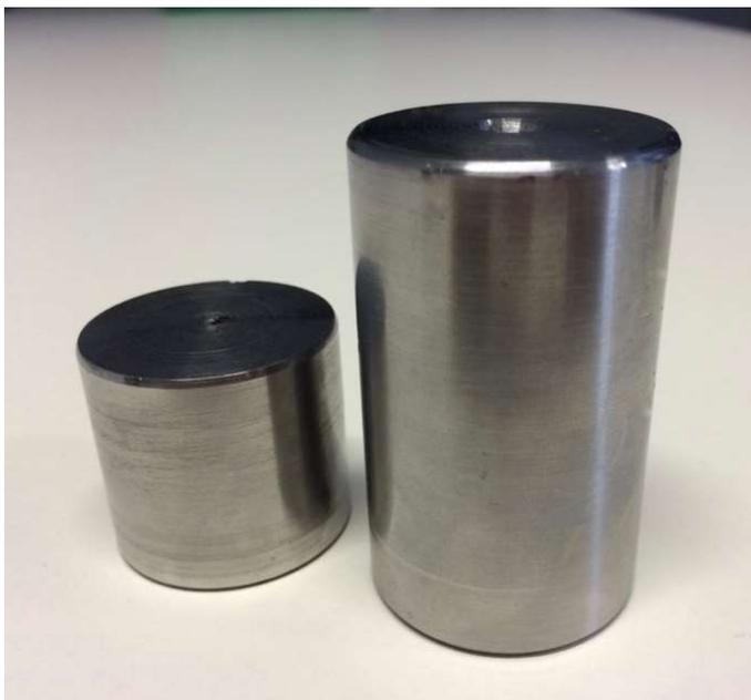
*Picture: Steel produced via the Matmor process*
