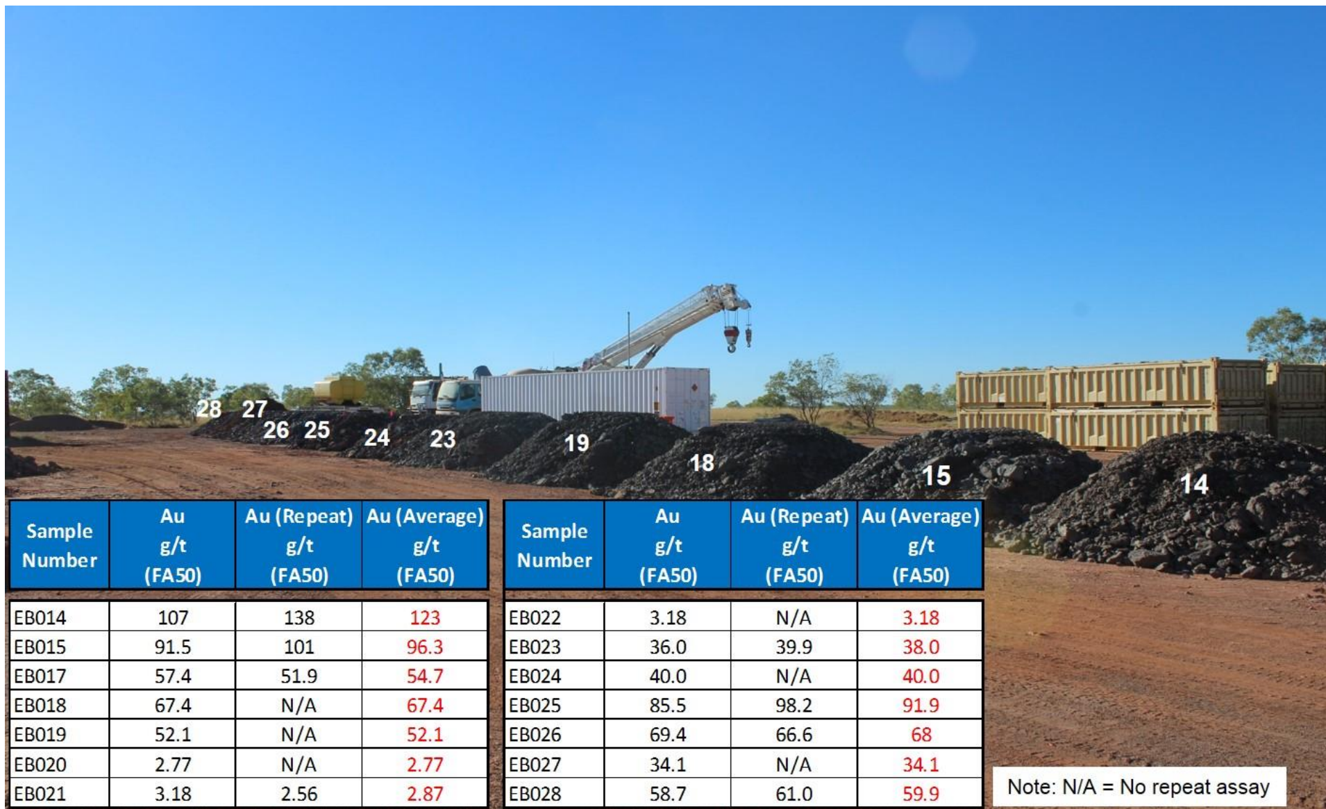
Figure 5: Development Ore on the ROM Pad at the Edna Beryl Mine. Note the gold assay results from the bulk samples
