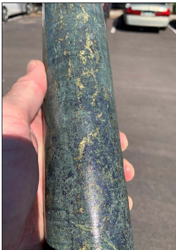
Core from drilling at the Talon. Mineralisation includes copper mineralisation with disseminated bornite (blue) and chalcopyrite (yellow) in skarnified sediments in drill hole WT-21-32 (272.1 to 272.5m) (refer ASX announcement 23 September 2021)
