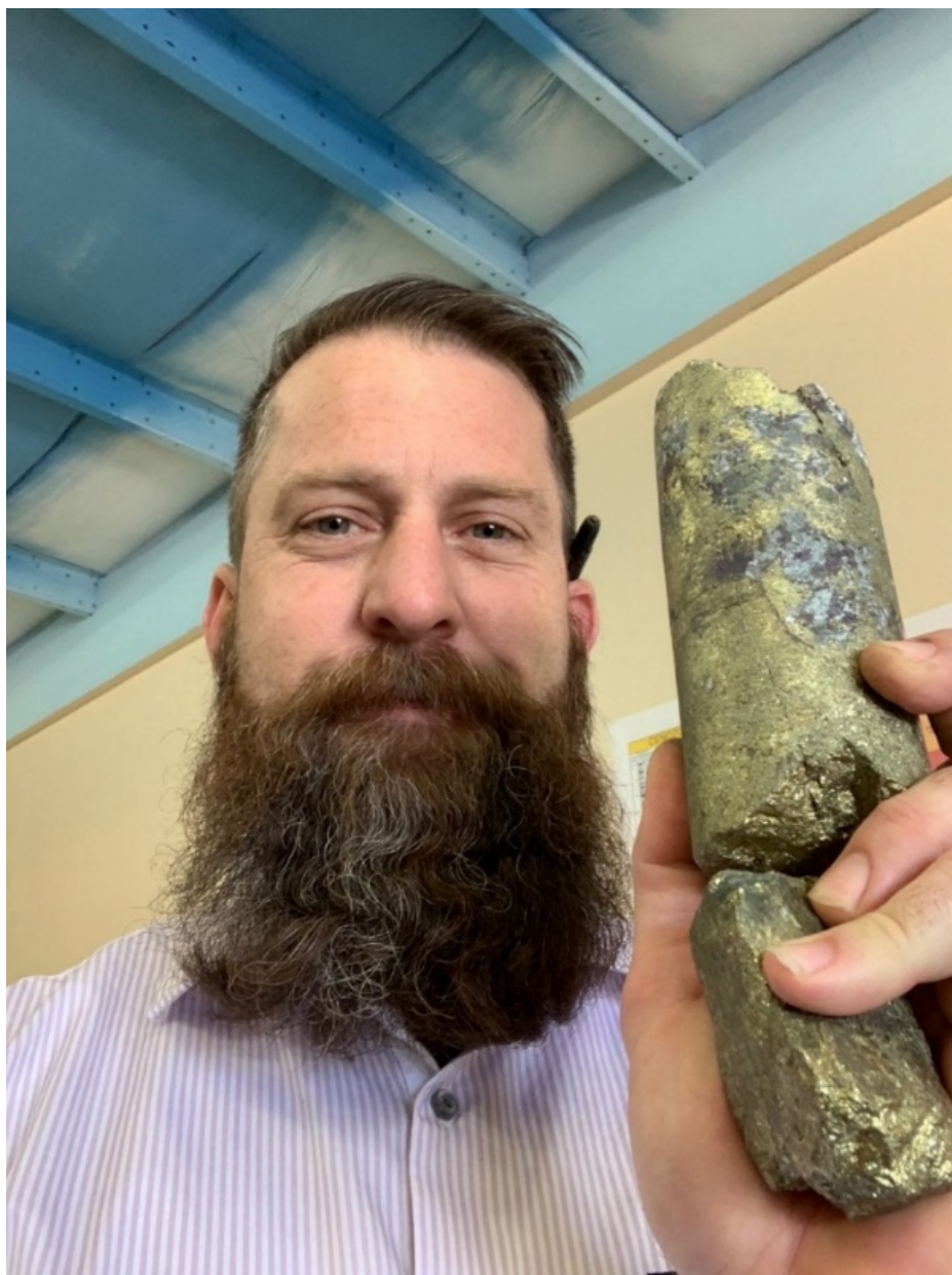
Principal Geologist Brian Paull holding core from WT-21-06 (from 371.6m) which assayed 34.4% Cu, 367g/t Ag and 26.2g/t Au (refer ASX announcement 31 March 2021).
