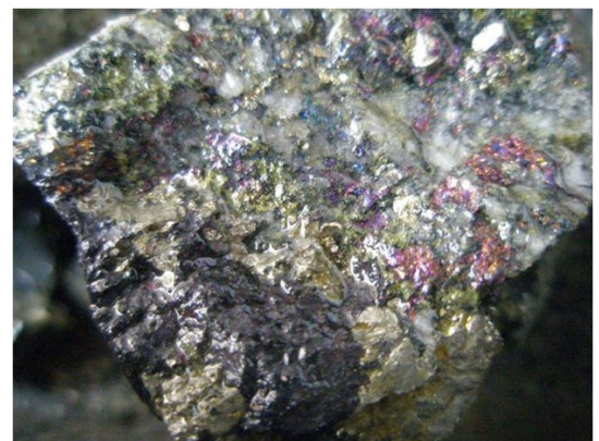
High grade Bornite-Chalcopyrite infilling veins, Calgoa prospect
