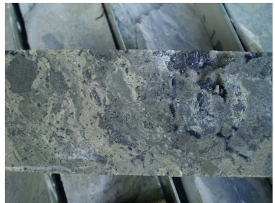
Late vuggy galena sphalerite veins 200m – 500m Hole BARD 1, Gayndah Prospect
