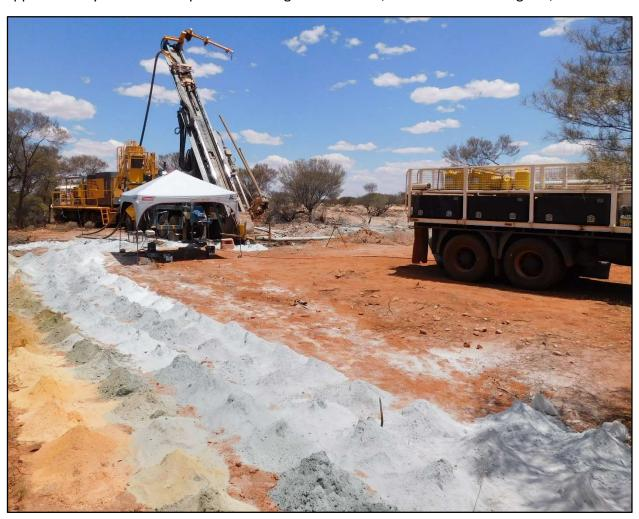
Image 1 - Eelya South Reverse Circulation drilling
