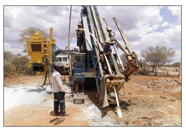
Image 2 - Installing PVC casing in 19ESRC013 for downhole geophysical surveys
