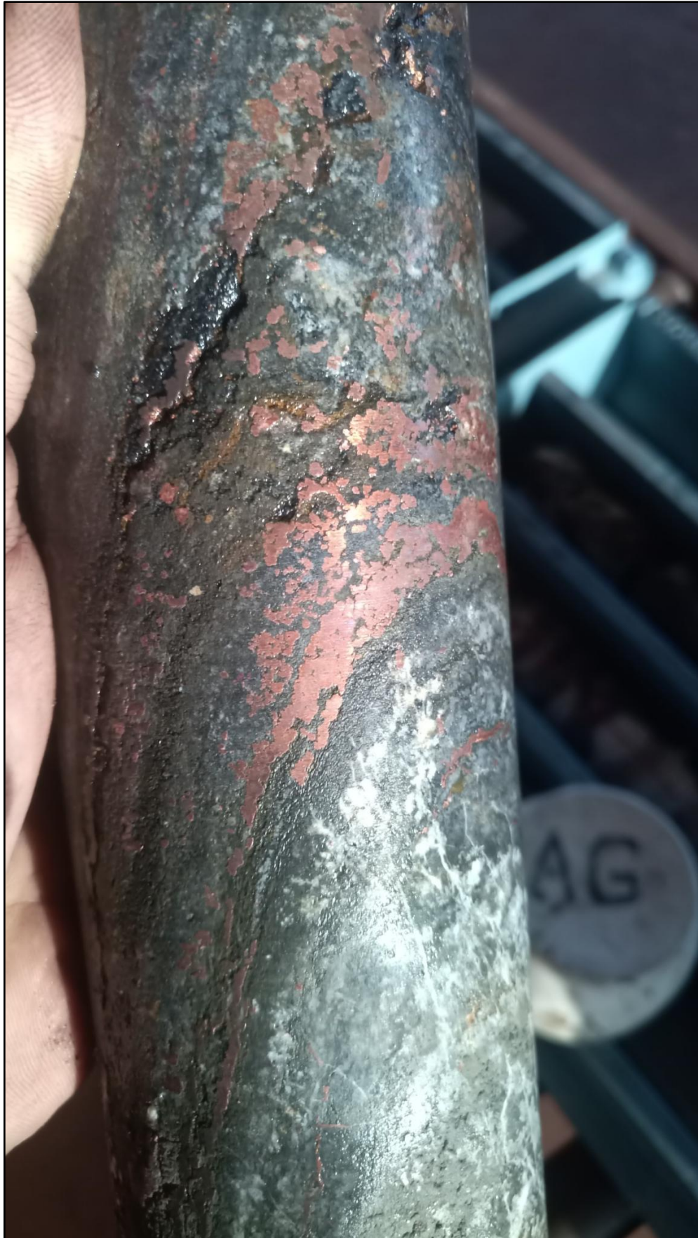
Figure 4 | Hole 21NDMT001: 150.3m to 150.5m showing native copper, covellite, chalcopyrite and chalcocite.
