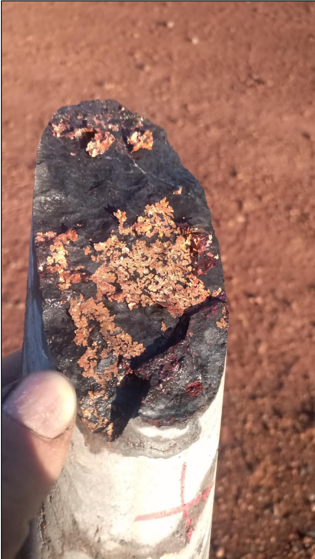
Figure 2 | Hole 21NDMT001: 141.4m to 141.5m showing native copper and chalcocite.
