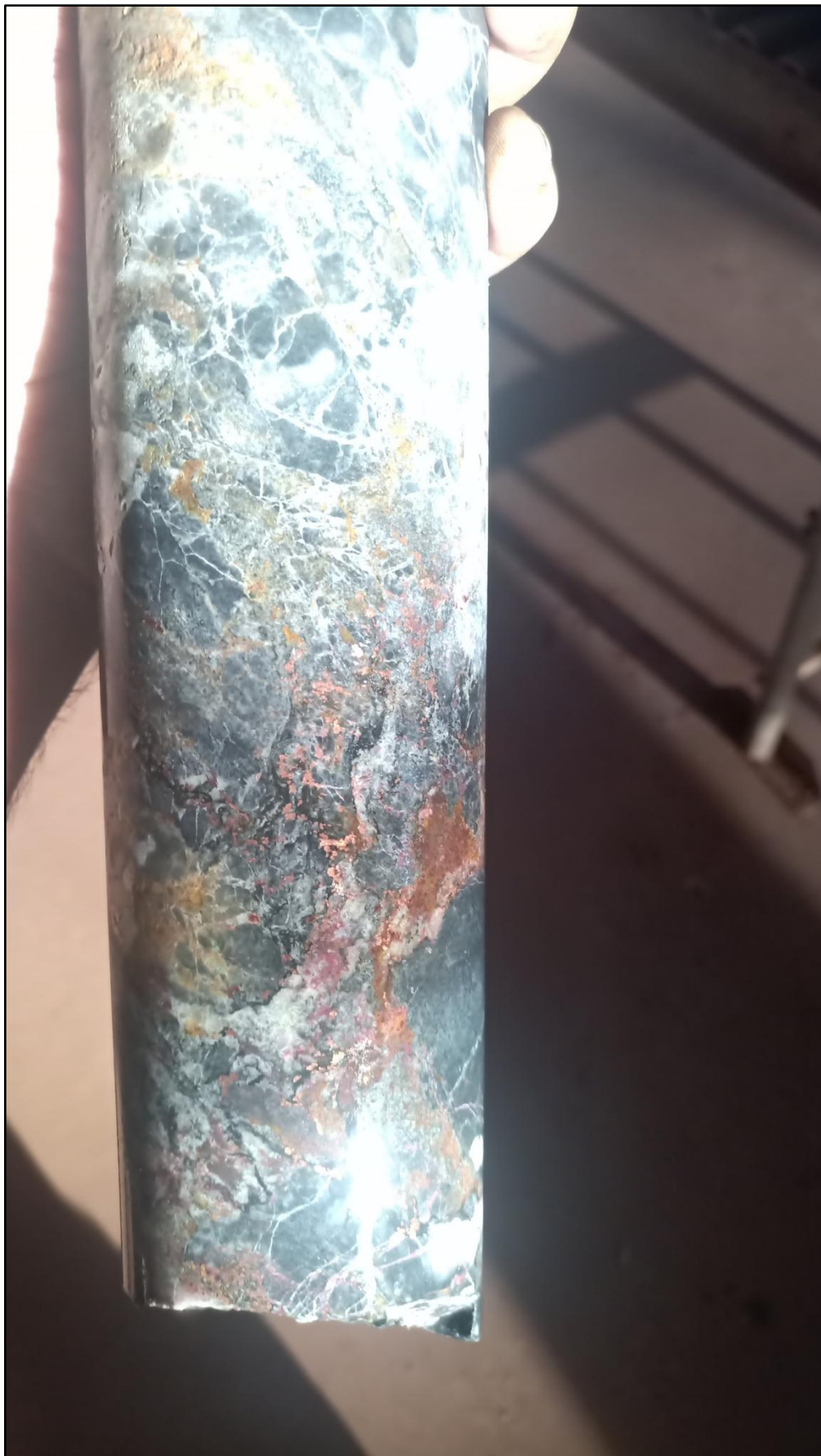
Figure 3 | Hole 21NDMT001: 148.2m to 148.4m showing native copper, covellite, chalcopyrite and chalcocite.
