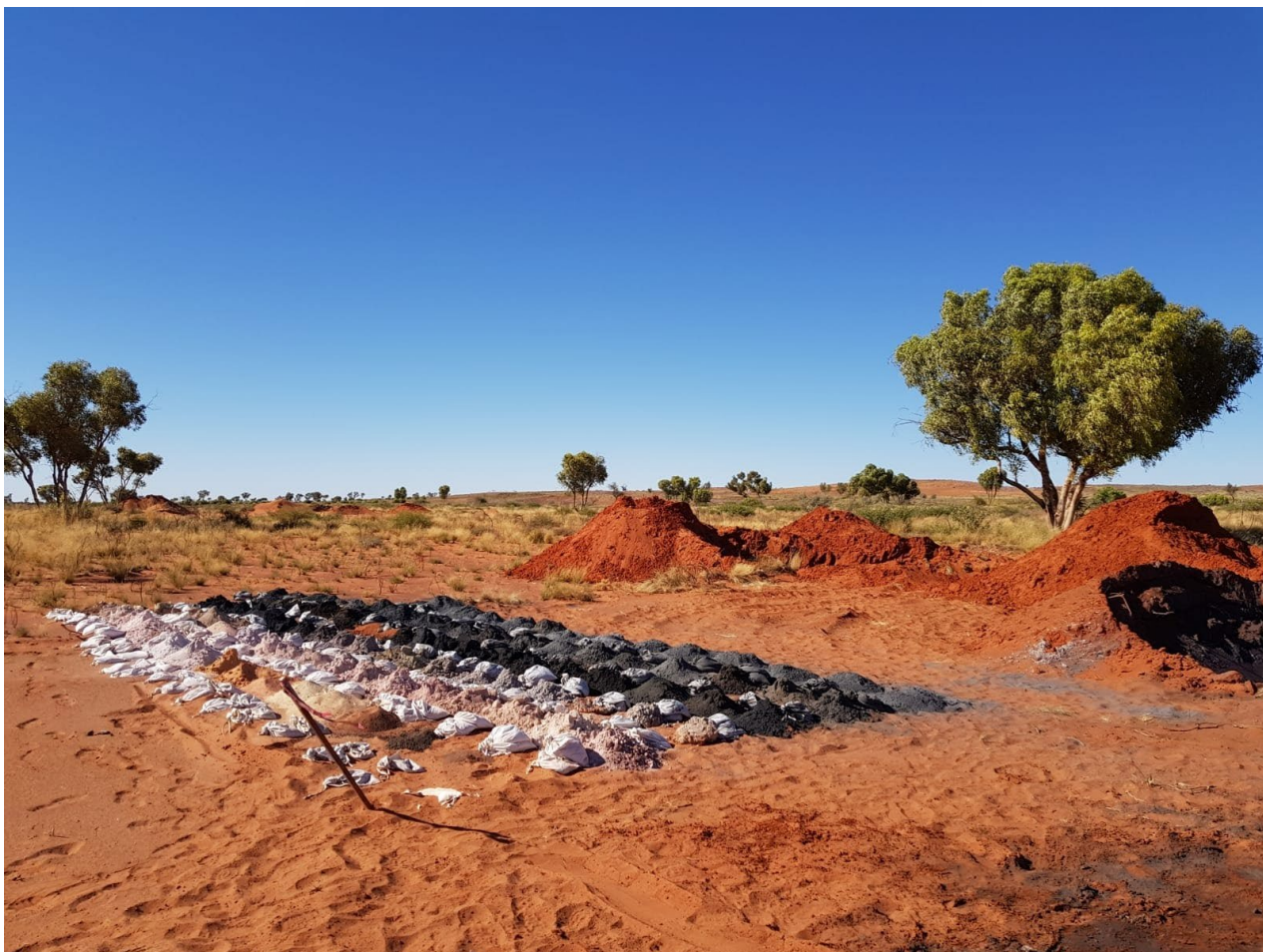
Figure 6 | RC drill samples from the third hole at Maroochydhore.
