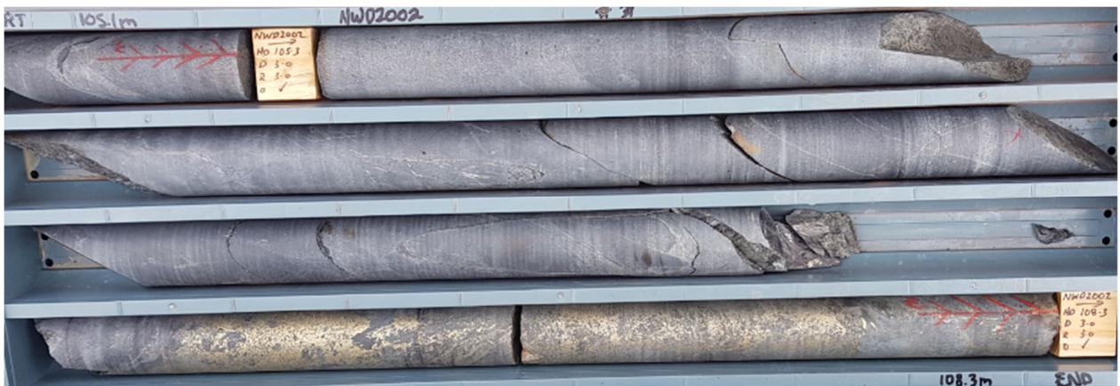
Image 3 | NWD2002 (drill core 107.5m to 108.0m downhole showing chalcopyrite and pyrrhotite mineralisation
