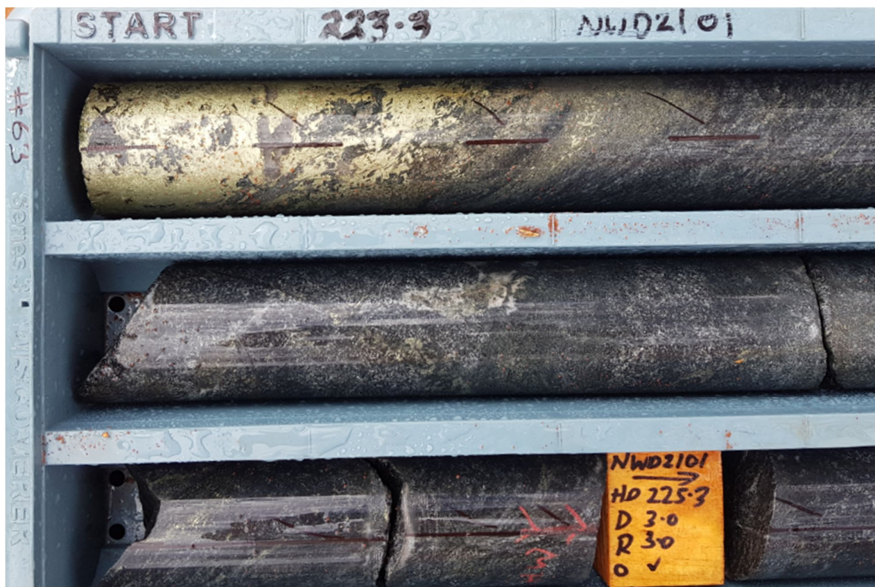
Image 11 | NWD2101 drill core 223.3m to 225.3m downhole showing chalcopyrite copper sulphide mineralisation
