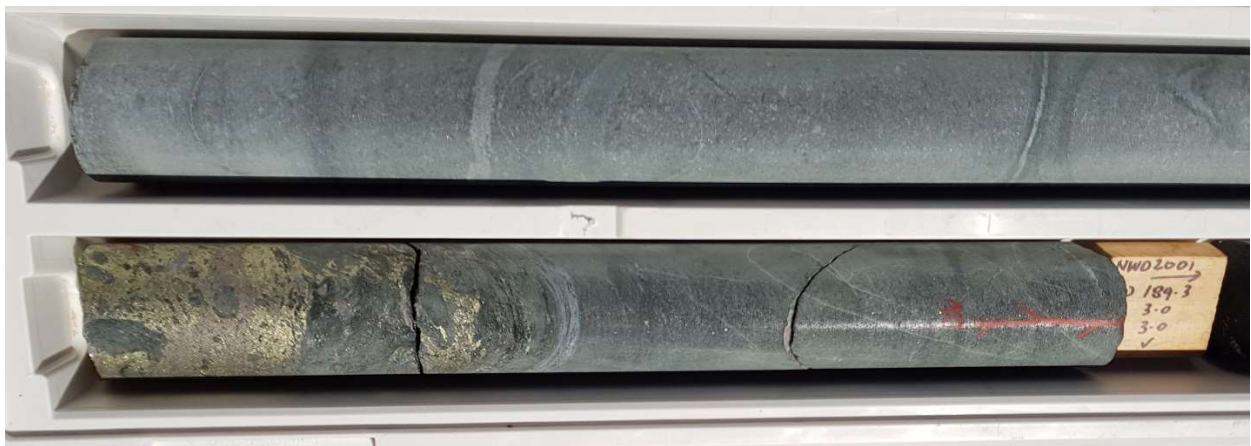
Images 2 | NWD2001 drill core 188.8m to 189.1m downhole showing chalcopyrite (yellow - copper sulphide) and pyrrhotite (bronze - iron sulphide) mineralisation
