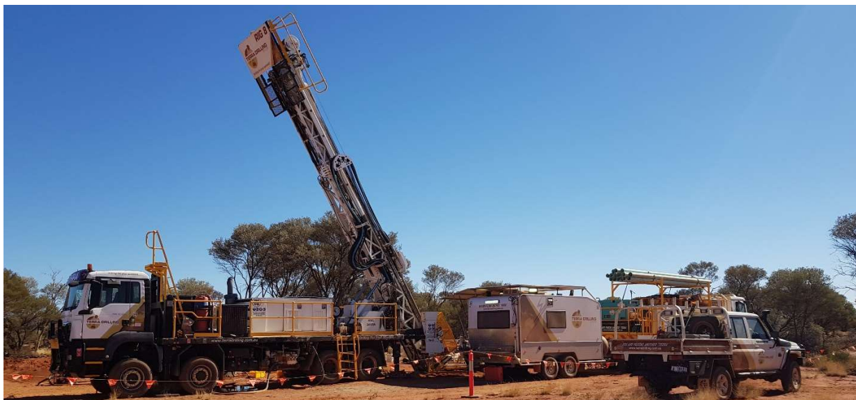
Image 5 | Diamond Drill Rig at Nanadie Well Copper-Gold Project
