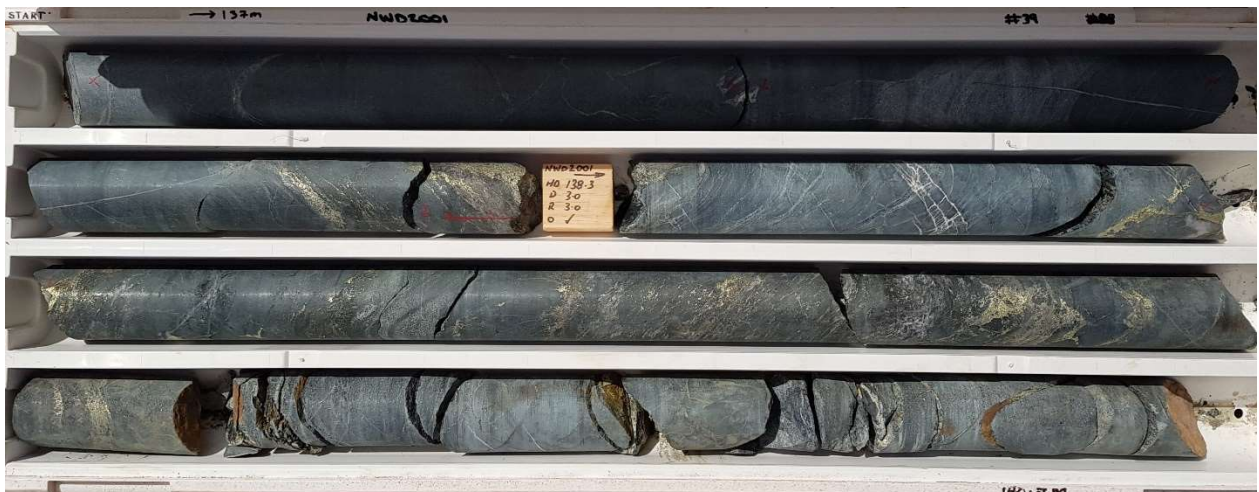
Image 1 | NWD2001 drill core 137.9m to 140.7m downhole showing chalcopyrite copper sulphide mineralisation
