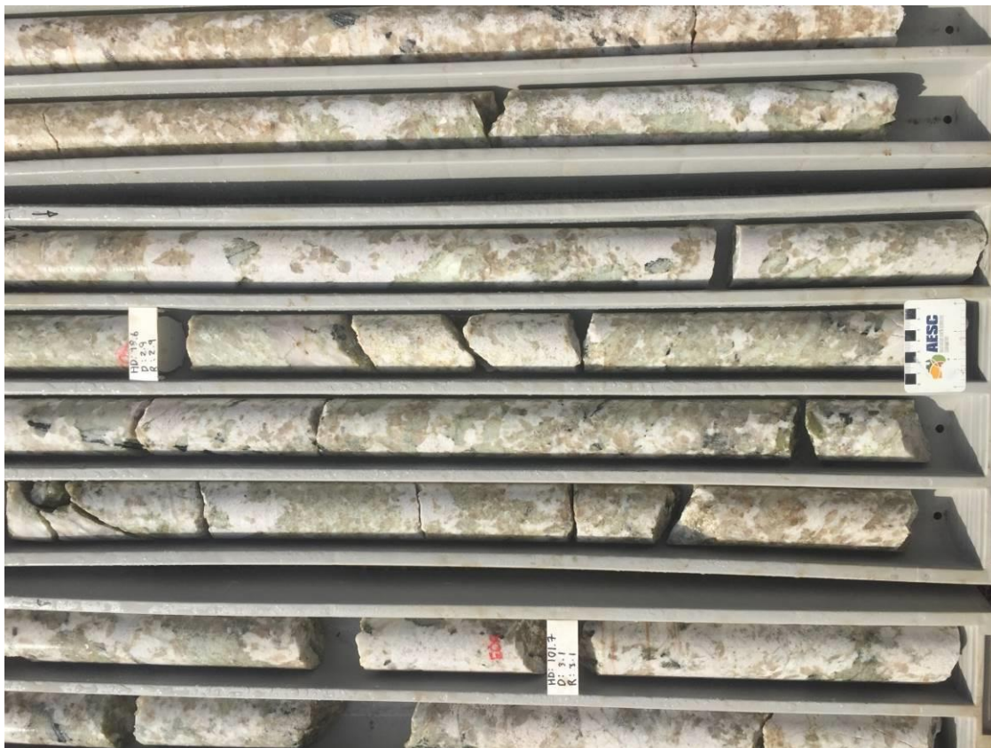
Figure 5. Large green spodumene crystals hosted by lighter coloured (white) feldspar and quartz. 95.2m – 103.1m FRDD001 (HQ), BP33 Prospect, Finnis Lithium Project NT.
