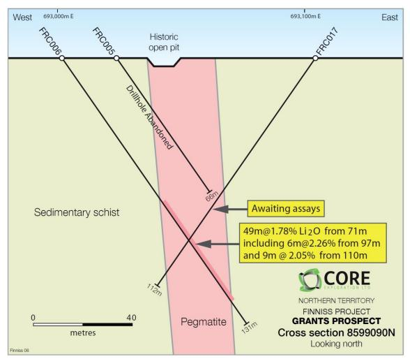
Figure 1. Cross section looking NE of Grants Pegmatite with recent RC drilling.
