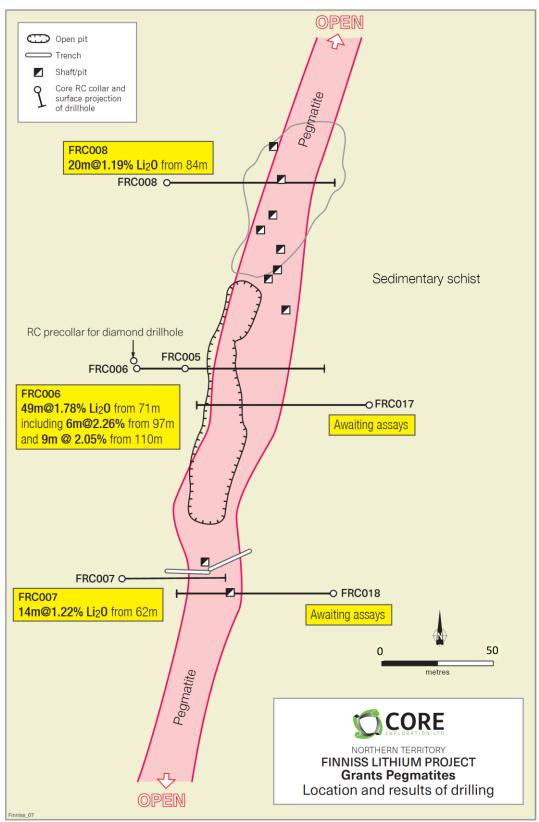
Figure 2. Grants Pegmatite showing Core's RC drilling and historic mining and trenching, Finniss Lithium Project, NT.
