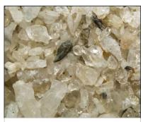
Test work Comp P100 5.6mm +0.5mm DMS100 SG 2.9 Overflow P100 3.35mm +0.5mm DMS100 SG 2.7 Overflow
