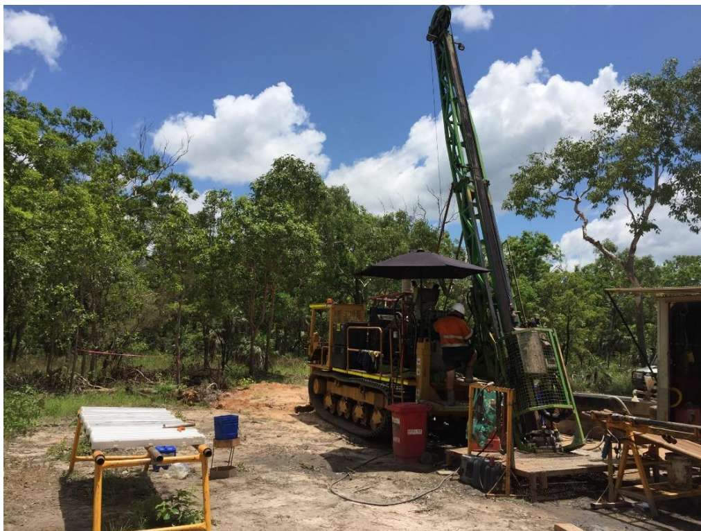
Figure 1. Diamond Drill Rig and Core at BP33, Finniss Lithium Project near Darwin in the NT.
