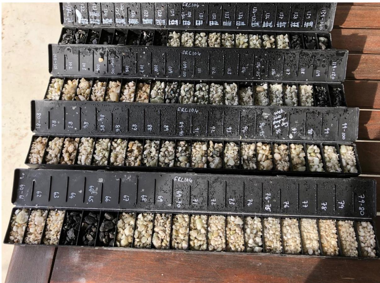
Figure 1. RC Drill chip tray D03 showing light colored spodumene pegmatite interval (Drillhole FRC104).
