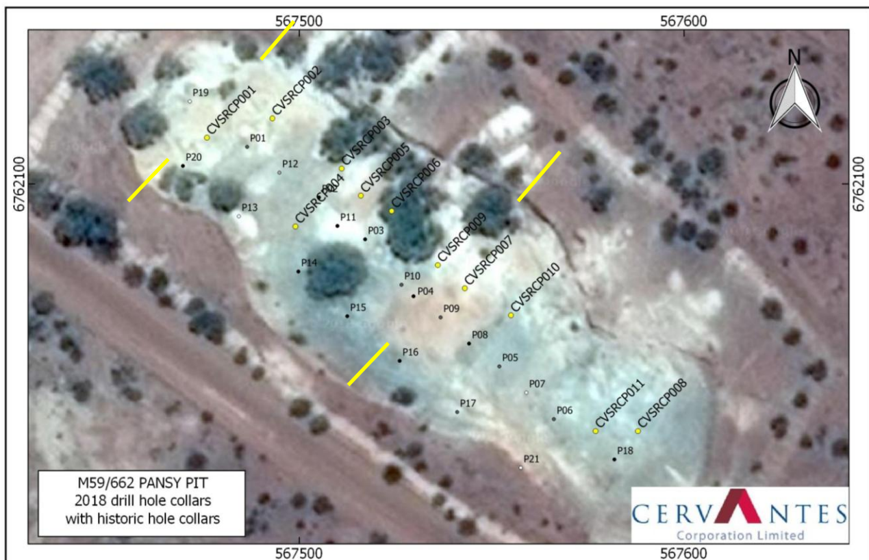
Figure 7: Collar locations in the Pansy Pit. The CVSRCP00x series are from the 2018 drilling campaign, the Pxx series are historic collars. All holes are drilled to the north west (40° TN) at a 60° dip. Location of cross sections indicated by yellow lines. Co-ordinate system is GDA94 Zone 50.
