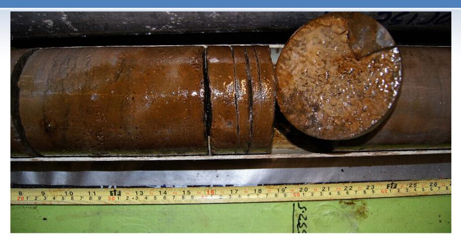
2551-2552m of 9m core Lower Stairway Sandstone-Surprise-1, Dec. 2010. 9m core zone alone assessed by RPS Energy capable of c.500-1,000 bbls/day, subject to confirmation by logging and pressure testing of visually obvious oil saturation.
