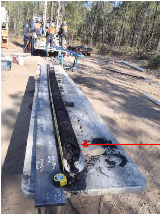
Coring by twinning open PCD hole ML002, the B9 seam is shown
