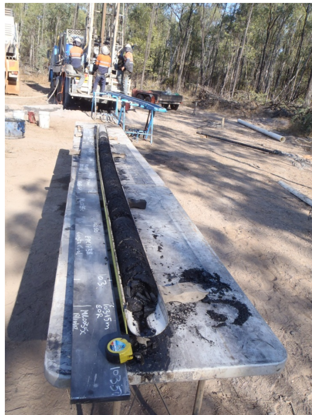
Figure 4: Coring by twinning open PCD hole ML002, the B9 seam is shown
