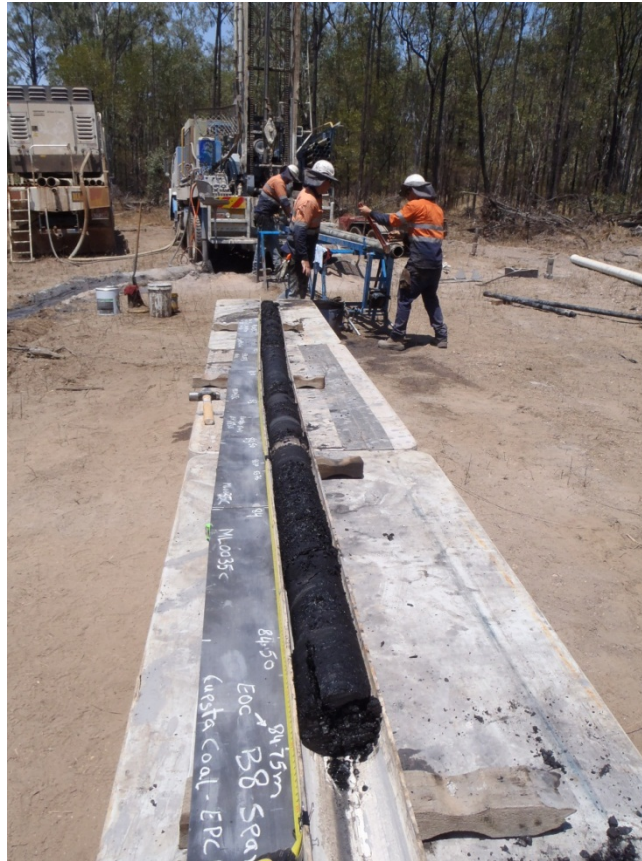
Figure 3: Coring by twinning open PCD hole ML002 a partial section of the B8 seam is shown
