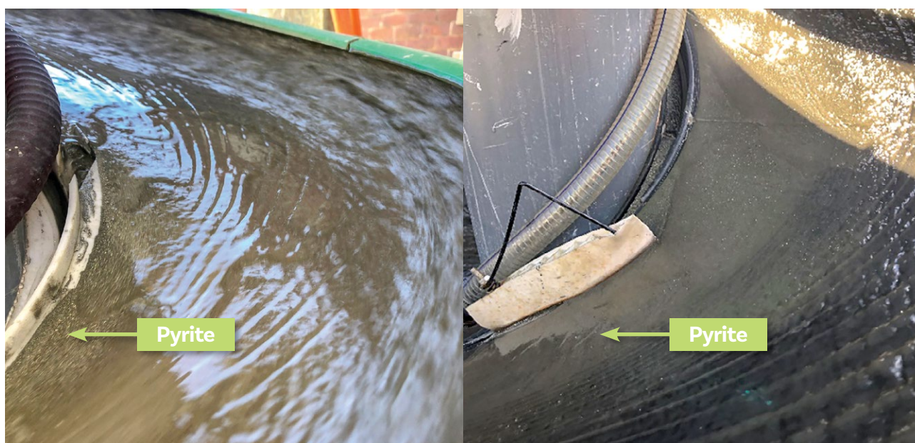
Figure 2. Operating rougher spiral (LHS) and cleaner spiral (RHS), with 'heavy' pyrite concentrate being separated from 'light' feldspar/silica gangue.
