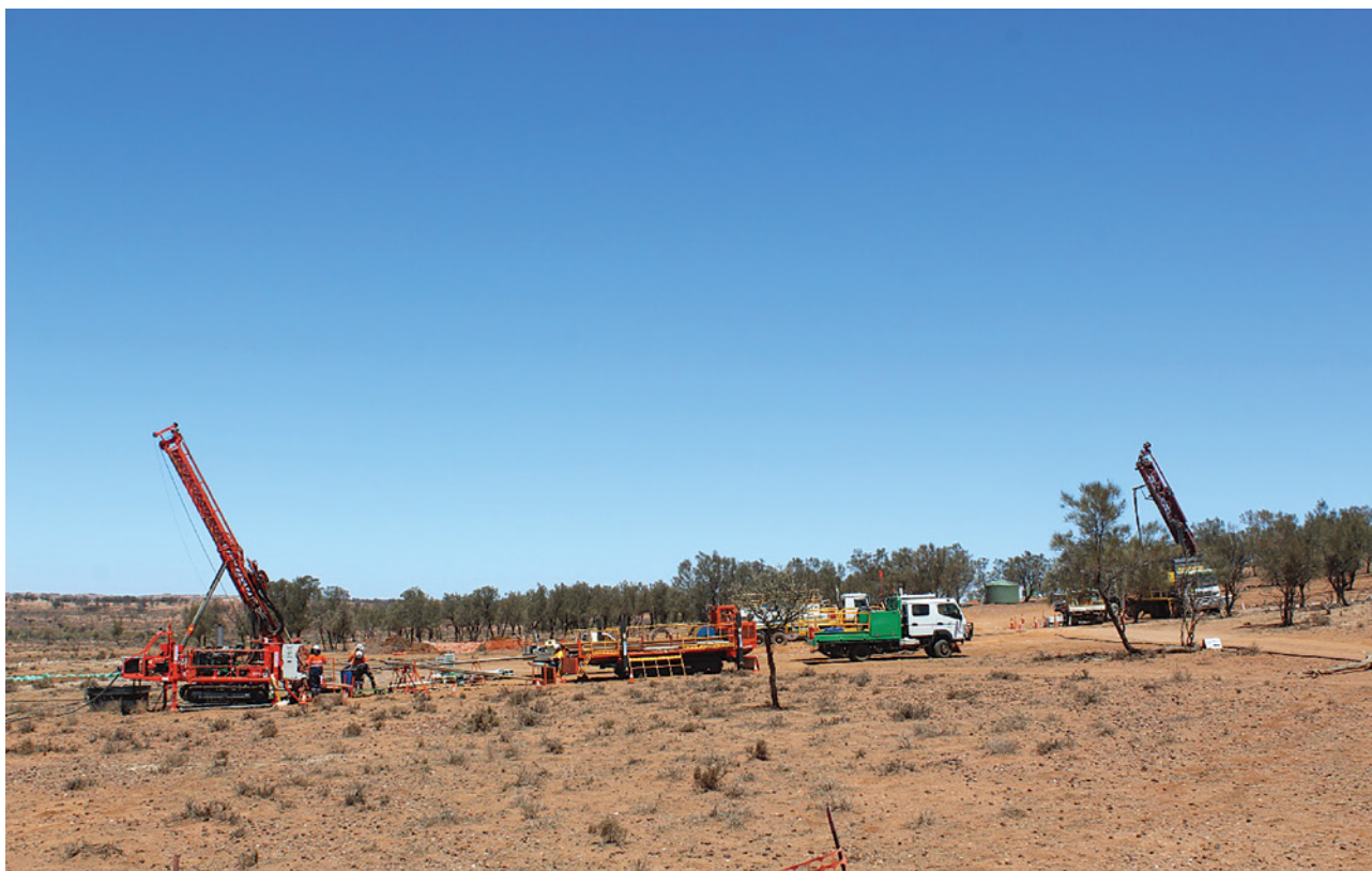
Figure 4. Reverse circulation and diamond drilling operations at Pyrite Hill.
