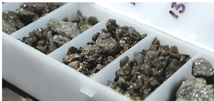
Figure 1. High grade pyrite mineralisation intersected during the current drilling campaign (assay results pending).
