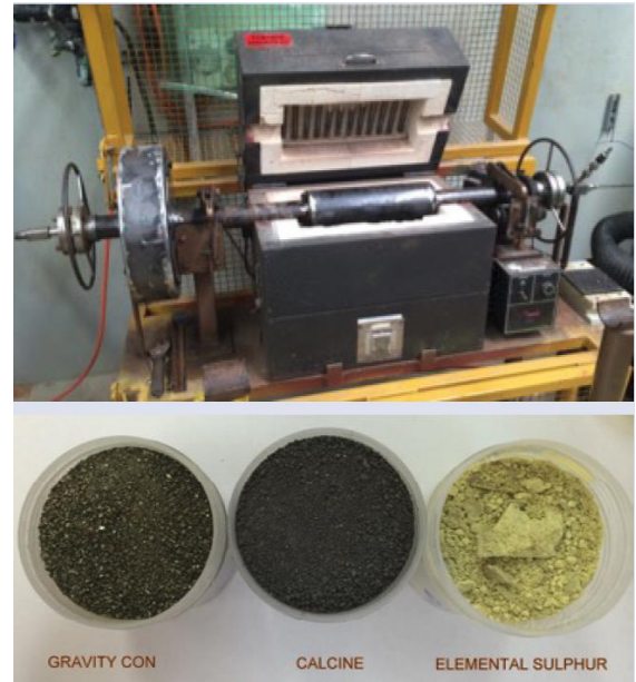
Above: Laboratory-scale furnace & elemental sulphur condenser. Below: Photos of the feed concentrate, residual calcine and collected elemental sulphur.
