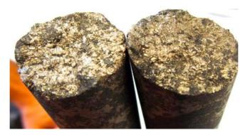
Image I: Drill core from Mammoth showing Semi massive & veined mixed sulphides in sheared mafic host
