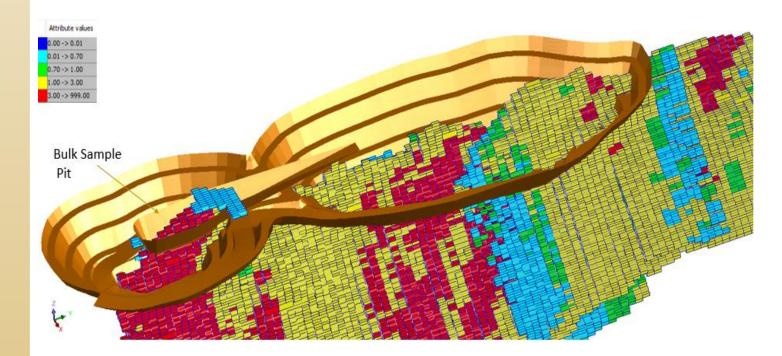
Figure 2 – Kat Gap Indicative Stage 1 Trial Open Pit Draped over Block Model (coloured by gold grade)
