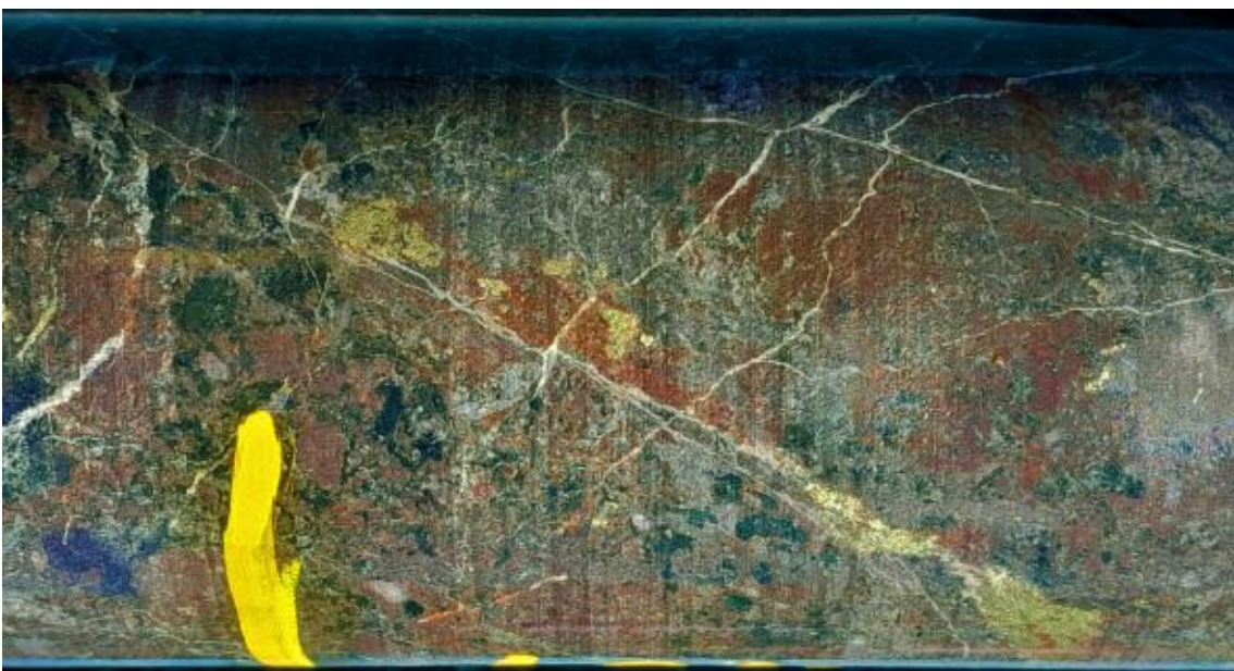
Figure 7: HWDD07 1157m. Vein and disseminated chalcopryite in altered mafic intrusive in the footwall of the upper Bluebush Fault.
