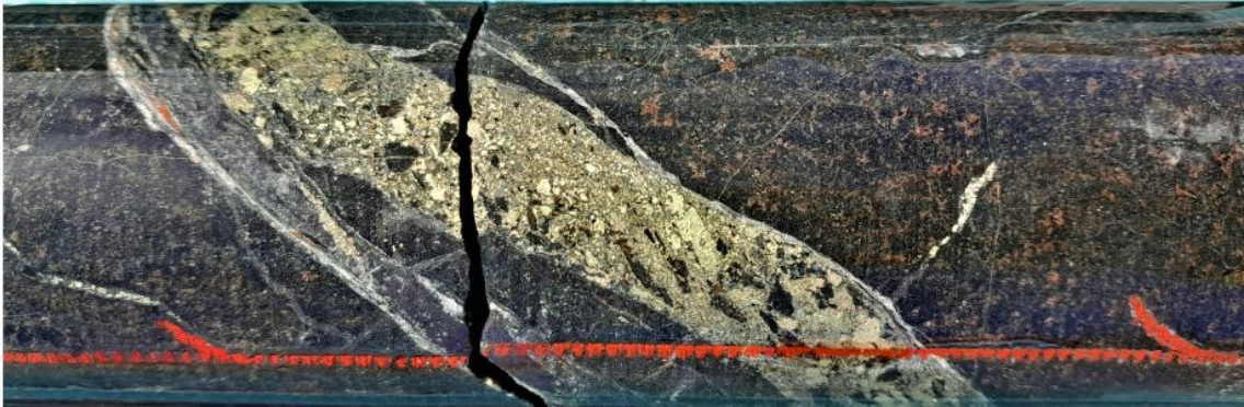
Figure 5: HWDD07 1350.4m Chalcopryite-Pyrite-Quartz vein in mafic intrusive.
