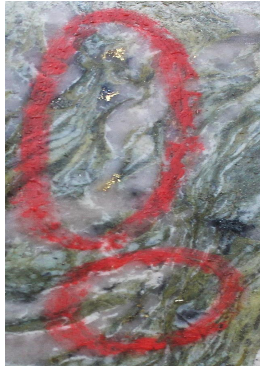
Visible gold within altered volcaniclastic drill core
