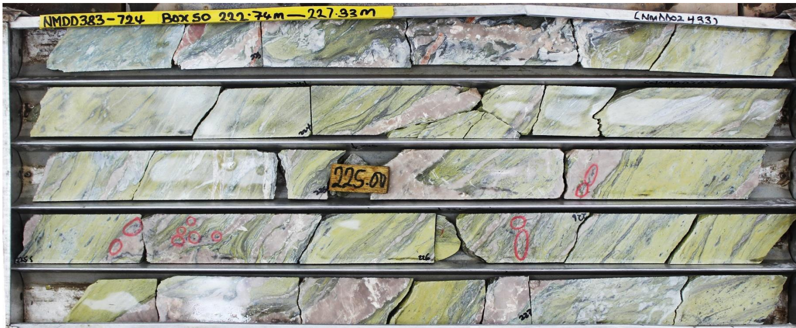
Cut drill core containing visible gold (red circles) within altered volcanoclastic rock unit
