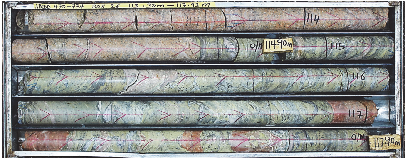
Figure 6: Mineralised volcaniclastics and granitoids within 50m @ 1.99 g/t Au zone (NMDD470-774)
