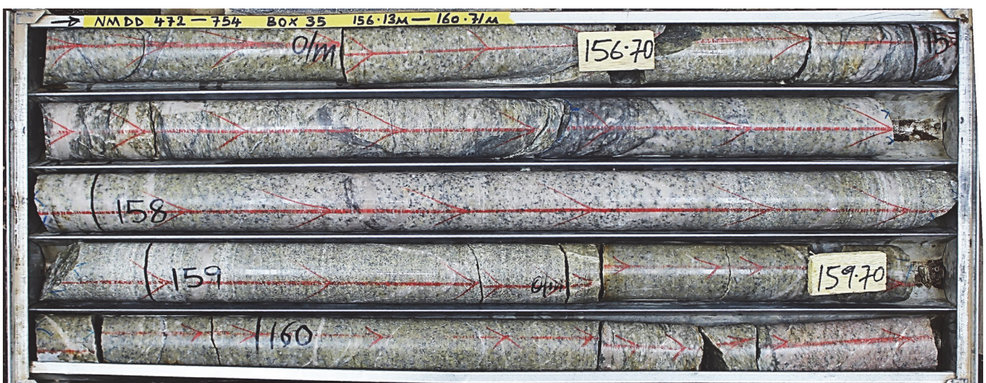
Figure 5: Mineralised granitoid within 58m @ 1.61 g/t Au zone (NMDD472-754)
