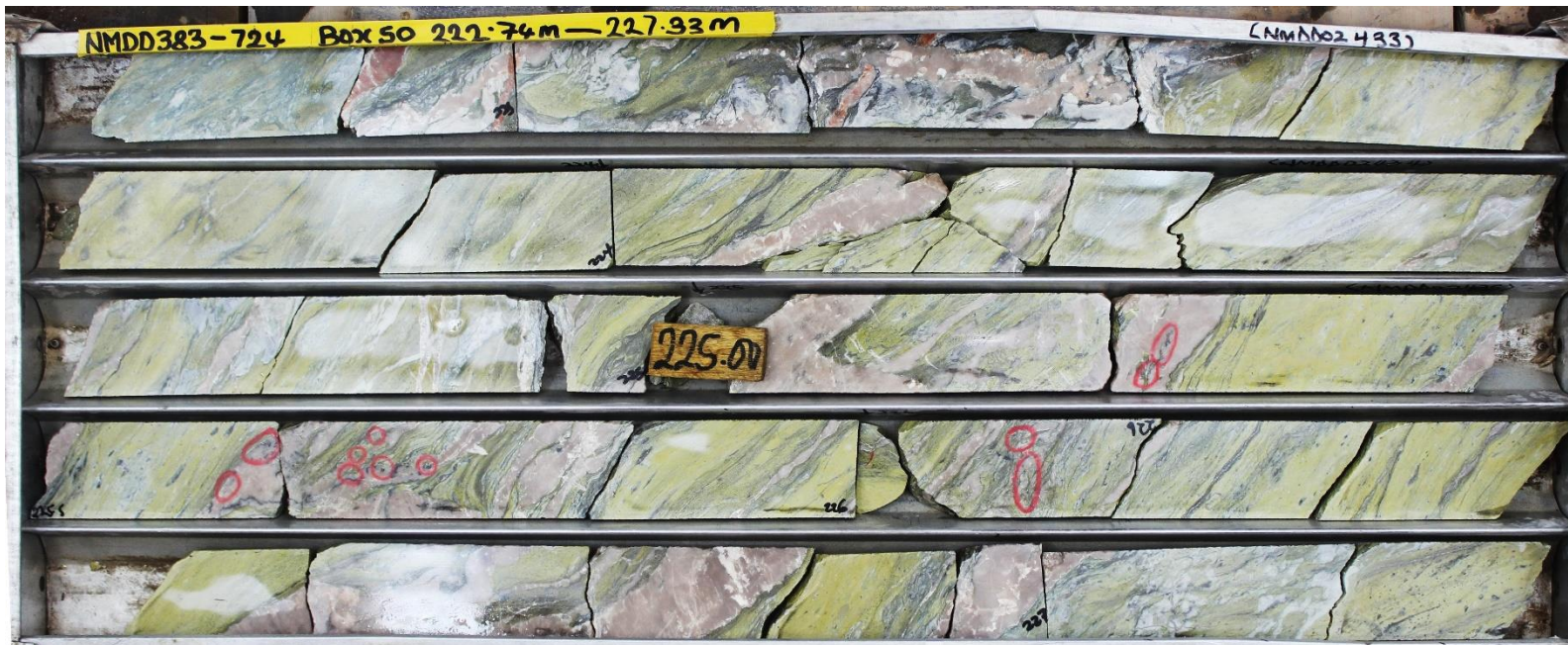
Cut drill core containing visible gold (red circles) within altered volcaniclastic rock unit
