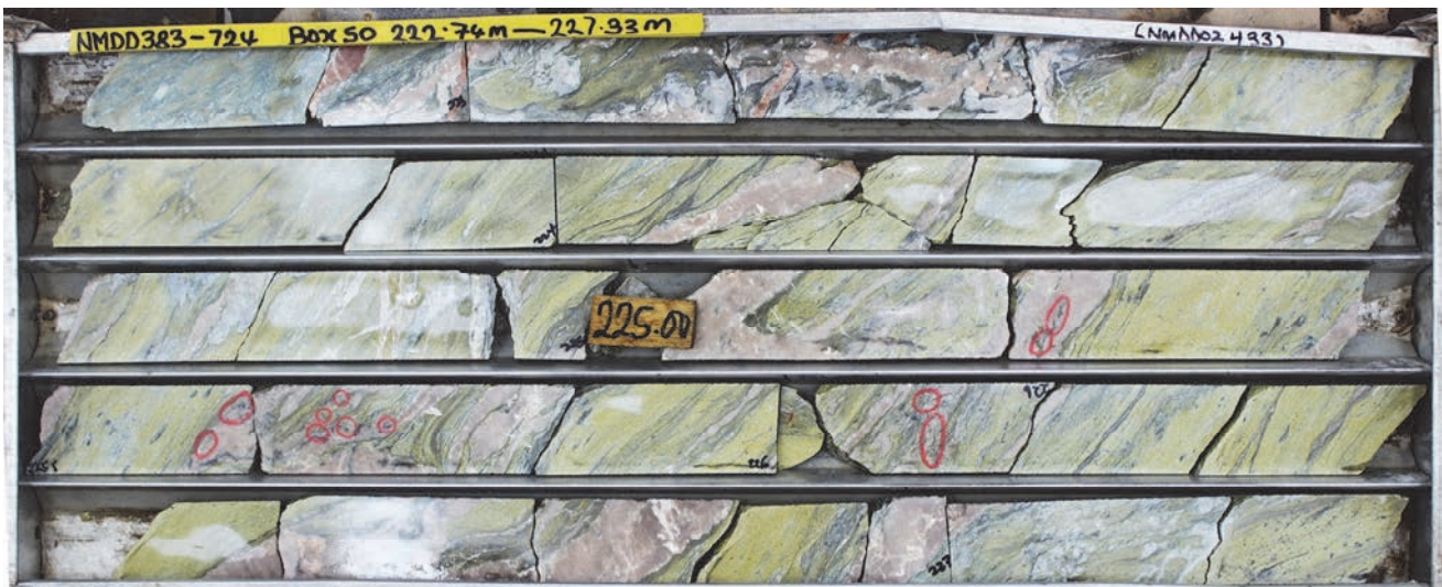
Figure 6: Altered volcaniclastic containing visible gold (red circles) between 225-227m (NMDD383-724)
