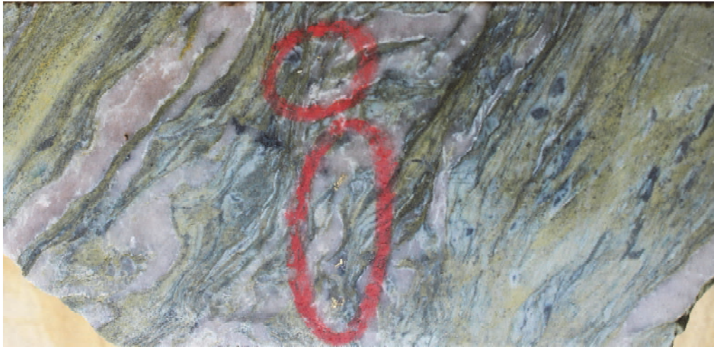
Figure 8: Altered volcaniclastic containing visible gold (red circles) between 226-227m (NMDD383-724)
